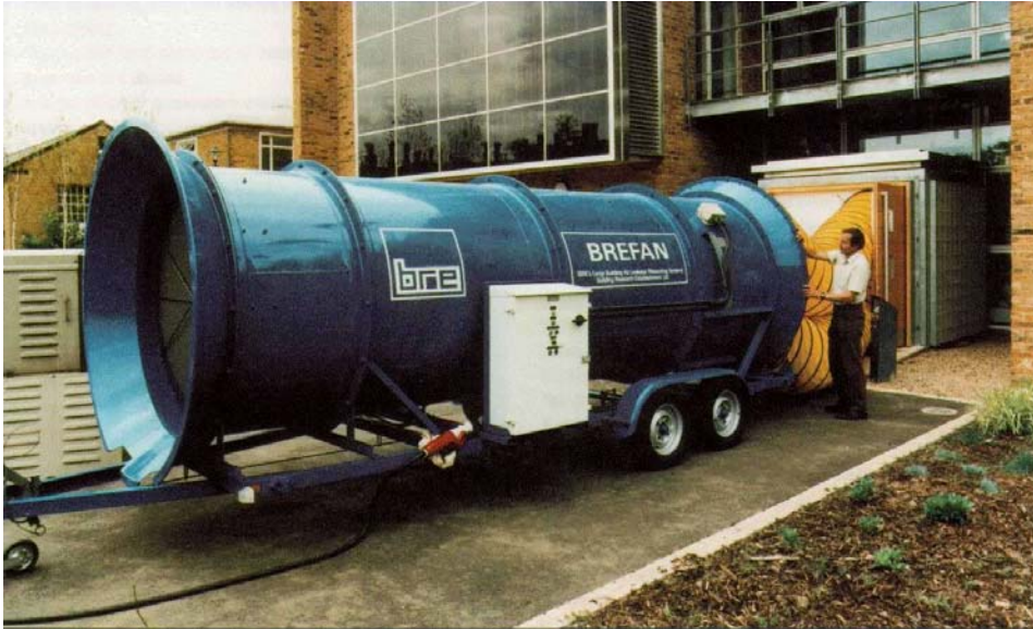
Figure 4.1: Photograph of fan system being used to test a building of 2000m 2 floor area. (Courtesy of BRE Watford UK).
