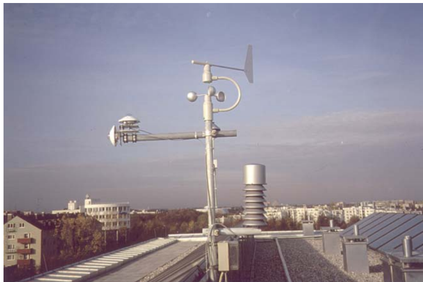
Figure 2.2.2: Weather stations should be mounted in an unobstructed position on the building or fairly close to it. The outside temperature and solar radiation need to be recorded.
