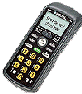
Figure 2.2.8: Pocketsized handheld computer and bar code scanner used for meter reading.
