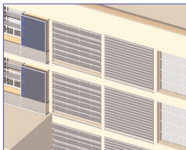
Combination of retrofitting interventions - light shelves, shading devices and PV panels
